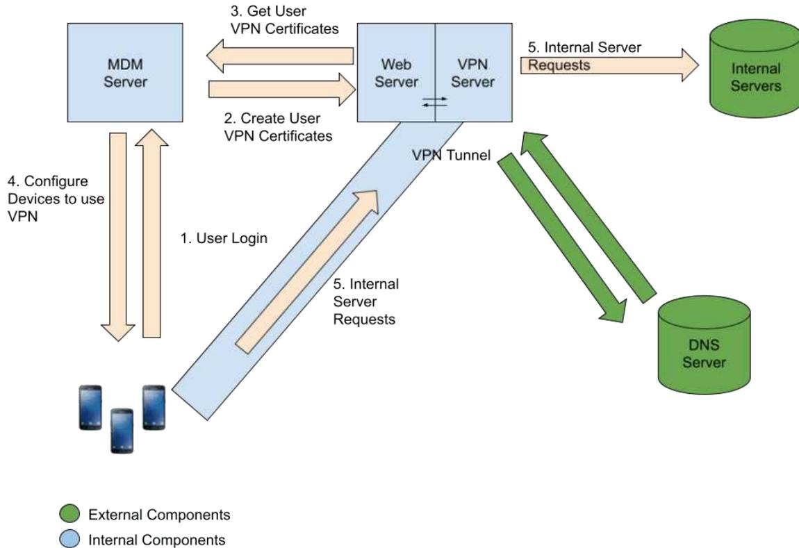
After the users log in on their devices, requests are sent from the MDM server to the Web and VPN servers for the creation of VPN-certificates. These confirm the certificates and send them back to the MDM server. The configurations are created in the admin interface and are sent to the devices. Afterwards, requests are sent via the VPN-tunnel to the internal servers. These requests differ from the VPN usage of the users.
